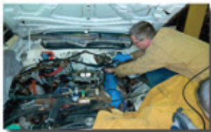
Tom Leahy inspecting and repairing valve cover gaskets.
