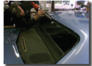
Mark Haga from Service Auto Glass installing the new back window
